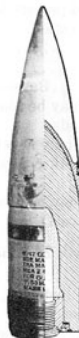
Figure 44. 6-inch Special Common Mk 27 Mods 1—8
