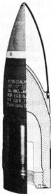
Figure 28. 5-inch Special Common Mk 38 Mods 1-3
